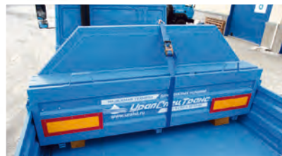
Mounting of the removable boards near the front side
