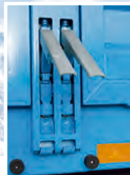
Locking mechanism on the removable racks
