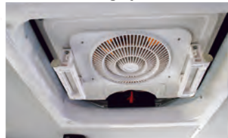
Radiator liquid heater connected to the engine cooling system
