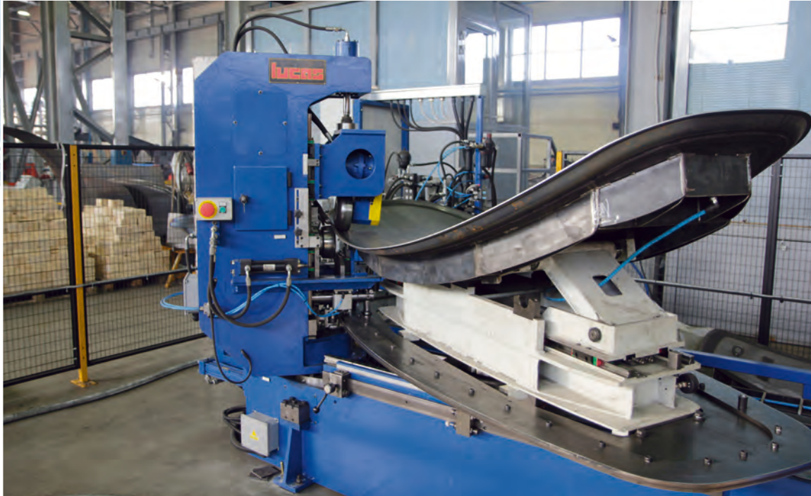
Machine for the manufacture of tanks bottoms
