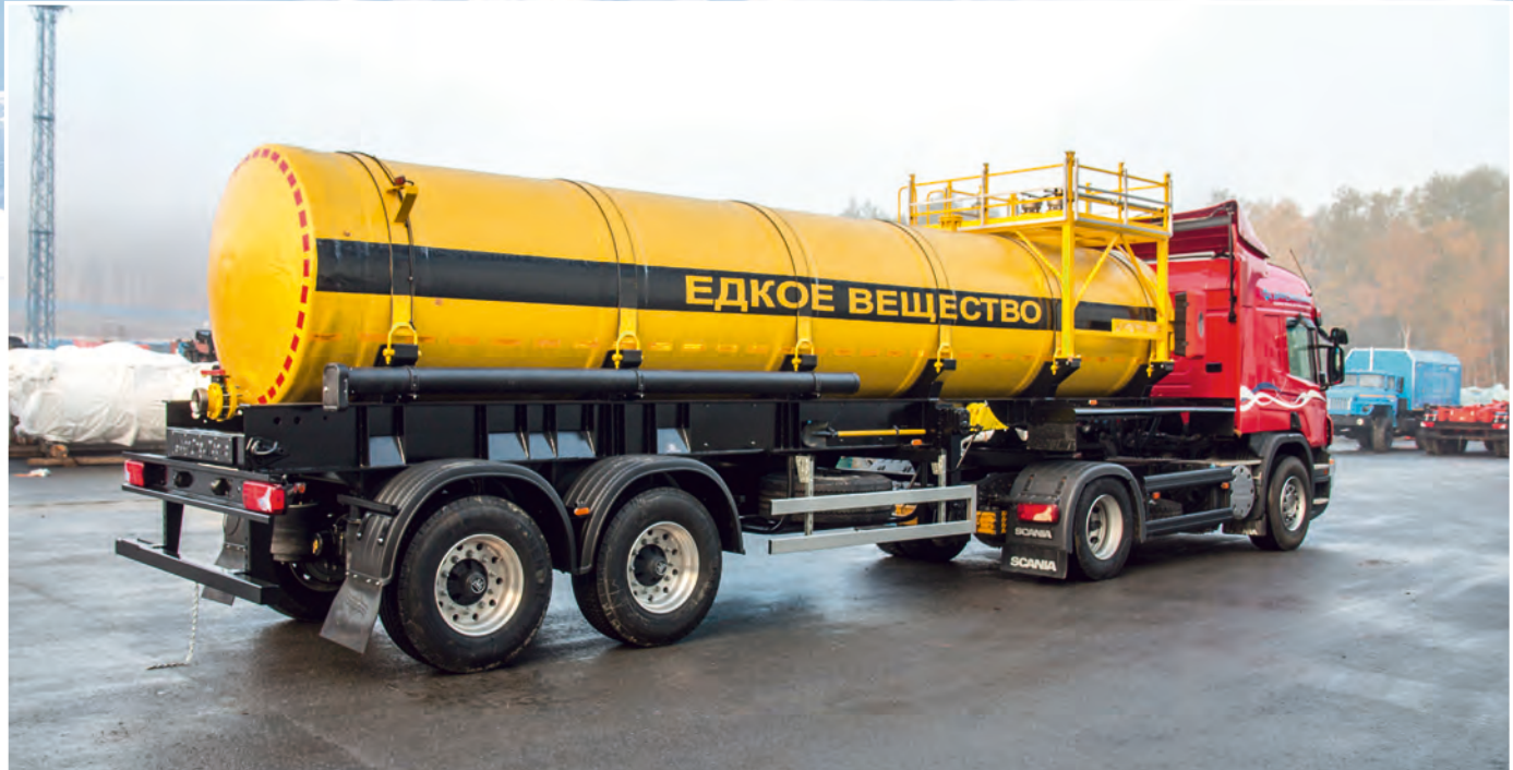
Tank from chemical resistant composite material to transport acid
