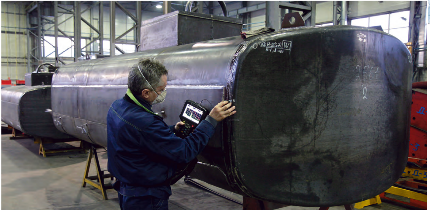
Quality control of welded seams of the tank using non-destructive ultrasonic testing
