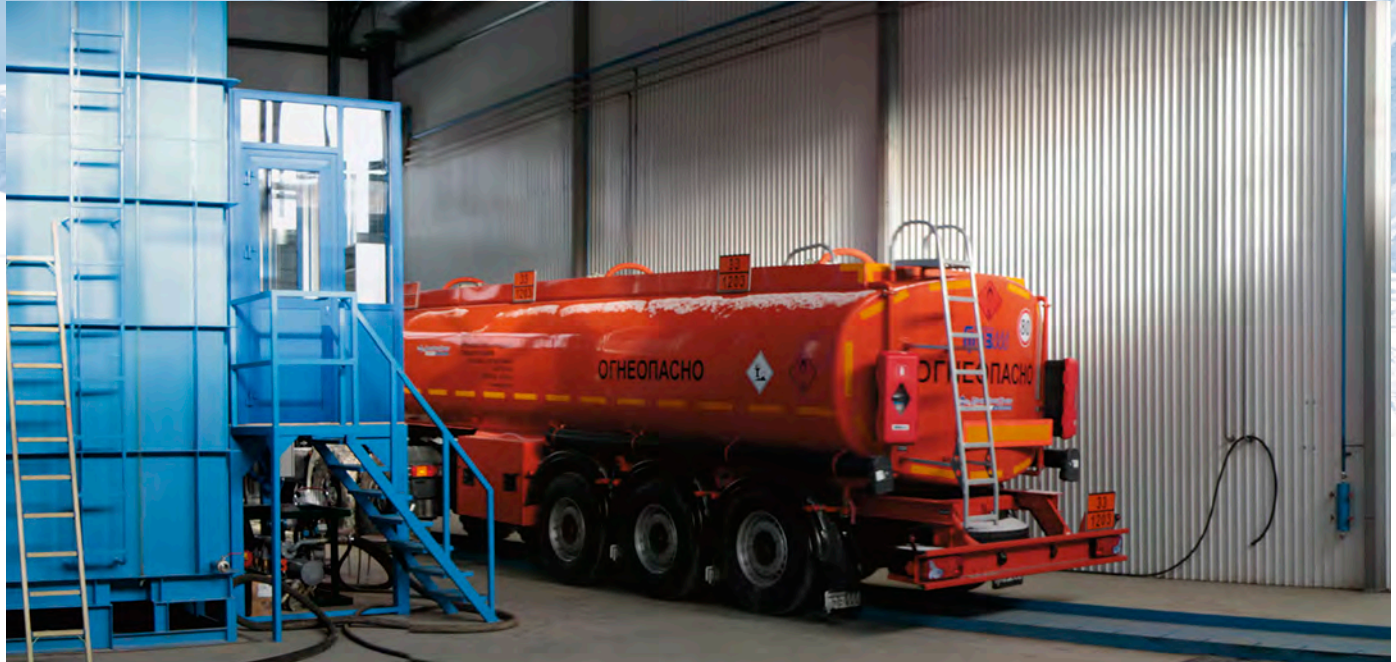
Equipment for calibration of the tanks with a certificate of calibration
