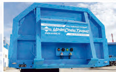
Reinforced front bar to protect the cab of the tractor
