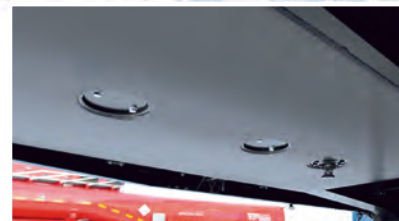
Mounting holes to install the pin with 3 position
