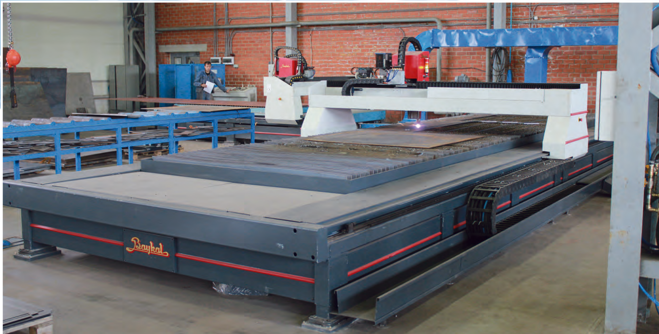
The equipment for plasma cutting
