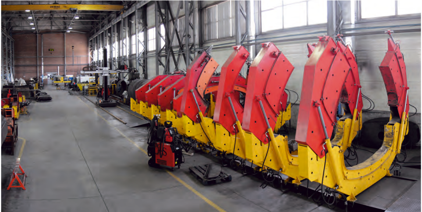
Equipment for forming of the tank
