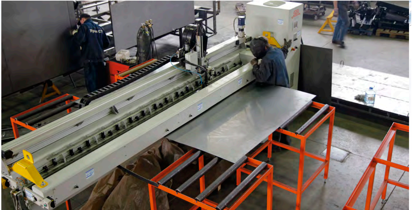
Equipment for welding of longitudinal seams
