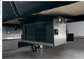
Radiator liquid heater connected to the engine cooling system
