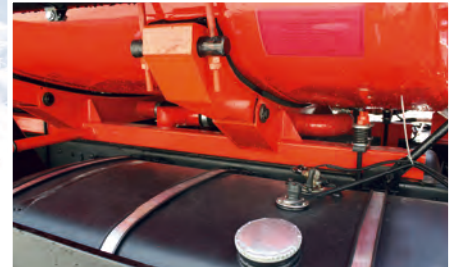
Lodgments, reinforcing plates, rubber damper
