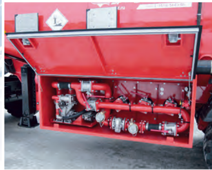
Fuel dispensing equipment
